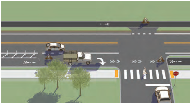
Figure 4-22. A variety of design treatments exist depending on the roadway configuration, available curb-to-curb width, traffic volumes and desire to provide a dedicated turn lane. All designs should strive to reduce speeds of turning vehicles, remind users of bicycle priority, and clarify user positioning up to and through the intersection.
