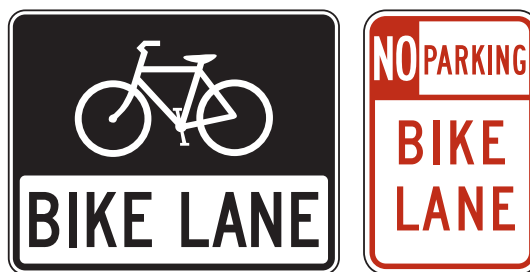
Figure 3-9. An optional R3-17 Bike Lane sign may be used to supplement bike lane markings. An R7-9 sign may be used if parked vehicles frequently block the bike lane.
