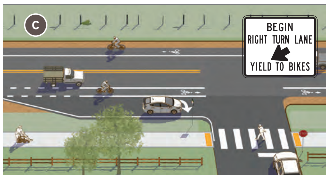
Figure 3-10. A variety of design treatments exist depending on the roadway configuration, available curb-to-curb width, traffic volumes and desire to provide a dedicated turn lane. All designs should strive to reduce speeds of turning vehicles, remind users of bicycle priority, and clarify user positioning approaching and through the intersection. Common signs at intersections include R4-4 Begin Right Turn Lane Yield to Bikes and a modified R10-15 Turning Vehicles Yield to Bikes sign. (1)
