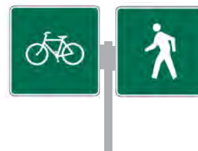
Figure 4-21. MUTCD signing options for specifying user types and path positioning can be used to indicate which users belong on the separate parts of a separated bike lane corridor (D11-1a, D11-2).
