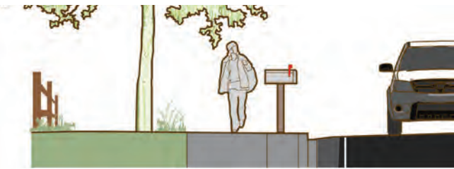
Figure 4-15. Sidewalks on roads with curbs may feature an unpaved or paved furnishing zone separation (left), or may be constructed with curb and gutter, immediately adjacent to the roadway (right). Offering separation from the roadway is preferred in most areas for user comfort and design flexibility at intersections.
